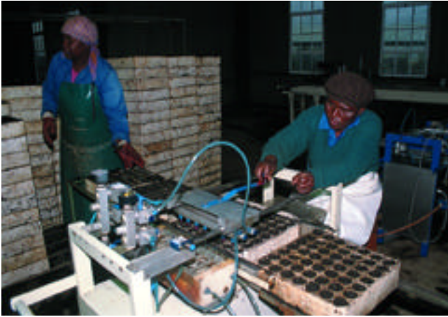
One of Sappi's workers uses a pneumatic device to place seeds in growing trays.
